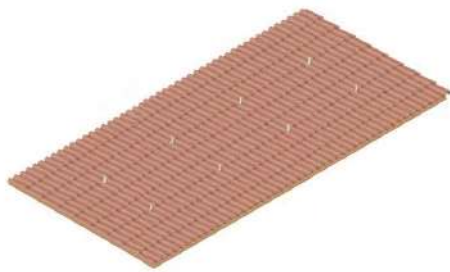
Step 3: Mount all the hooks with spacing as specified in the drawing with good alignment
