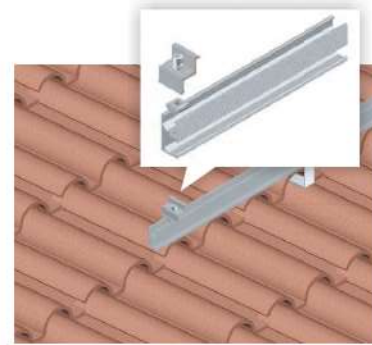
Step 5: Fix the 1st end clamp but not tighten at location as specified in the drawing
