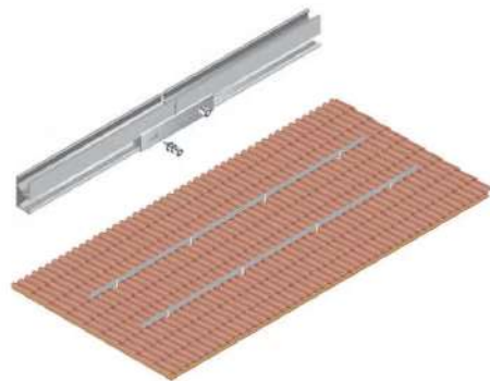
Step 4: Secure the rail on the hooks
